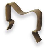
Mounting clips facilitate the safe and efficient mounting of semiconductors to heatsink with the corresponding hole pattern. Especially for insulated mounting, a clip provides reliability by making screws and insulation bushes dispensable. Central contact pressure distributes the heat conductivity equally across the semiconductor/hestsink contact surface.
