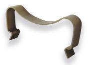
Mounting clips facilitate the safe and efficient mounting of semiconductors to heatsink with the corresponding hole pattern. Especially for insulated mounting, a clip provides reliability by making screws and insulation bushes dispensable. Central contact pressure distributes the heat conductivity equally across the semiconductor/hestsink contact surface.
