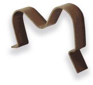
Mounting clips facilitate the safe and efficient mounting of semiconductors to heatsink with the corresponding hole pattern. Especially for insulated mounting, a clip provides reliability by making screws and insulation bushes dispensable. Central contact pressure distributes the heat conductivity equally across the semiconductor/hestsink contact surface.
